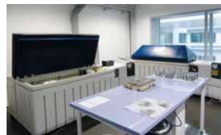
Fig. 13: Picture from our corrosion lab with various corrosion testing chambers.
