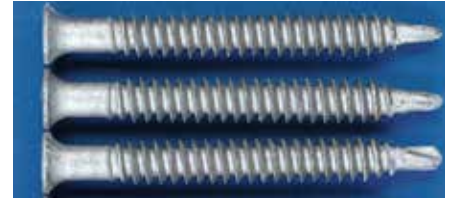
Fig. 20: Screws with highly corrosion-resistant multilayer coating after 15 cycles of the sulfur dioxide corrosion test (showing no corrosion).
