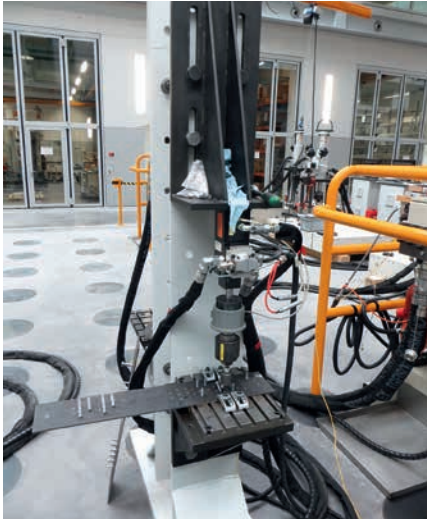
Hilti S-BT HL fastening system under cyclic loading
