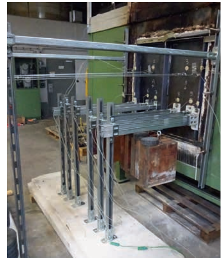
Figure 2: Test facility for fire test (small bulkhead)
