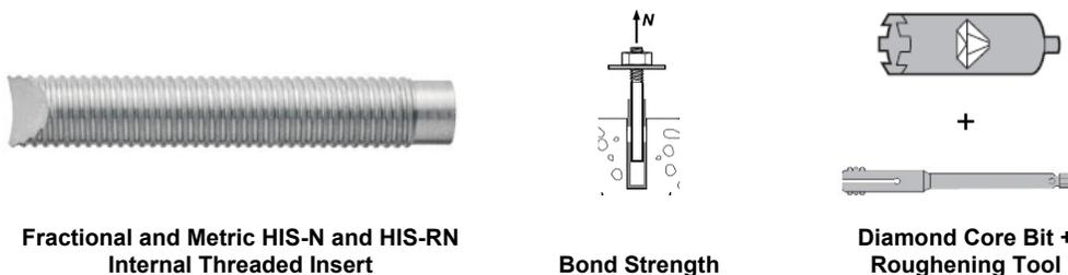
**TABLE 29—BOND STRENGTH DESIGN INFORMATION FOR FRACTIONAL AND METRIC HILTI HIS-N AND HIS-RN INSERTS IN HOLES CORE DRILLED WITH A DIAMOND CORE BIT AND ROUGHENED WITH A HILTI ROUGHENING TOOL<sup>1</sup>**
