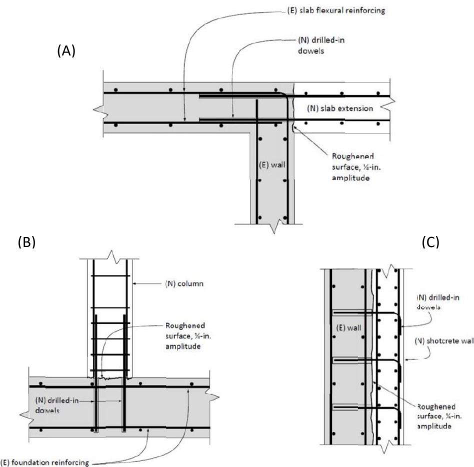
FIGURE 3—(A) TENSION LAP SPLICING WITH EXISTING FLEXURAL REINFORCEMENT; (B) TENSION DEVELOPMENT OF COLUMN DOWELS; (C) DEVELOPMENT OF SHEAR DOWELS FOR NEW ONLAY SHEAR WALL
